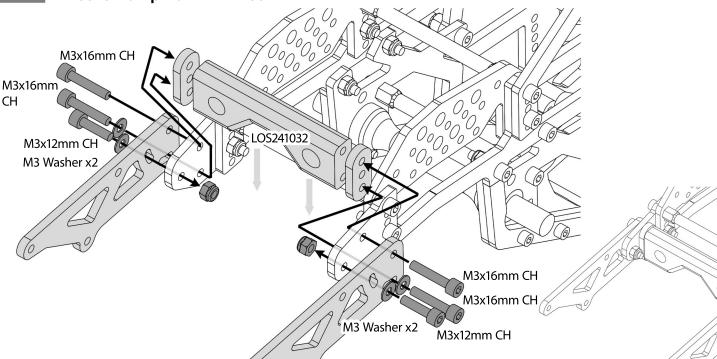
1. Install TLR Tuned LMT Wheelie Bump Bar TLR141001. 2. Install Battery Straps.
